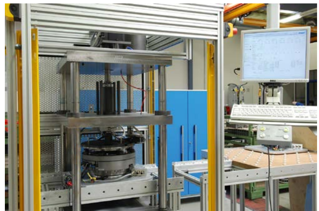
100 % quality: Before delivery, every single brake is checked and the results are recorded.
