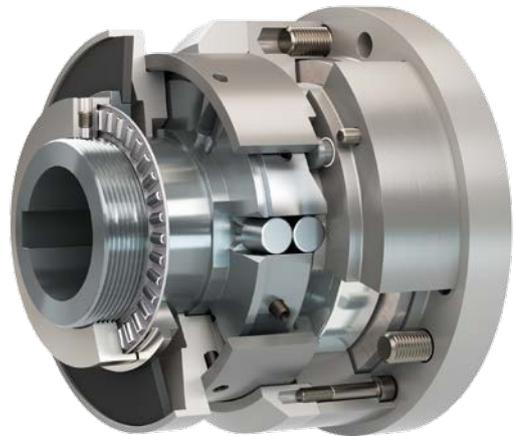
**On the EAS<sup>®</sup>-reverse, the use of cup springs with a negative characteristic curve causes an instant drop in torque. This prevents the so-called pumping or breathing of the clutch. This generates low wear on the disengagement mechanism.**
