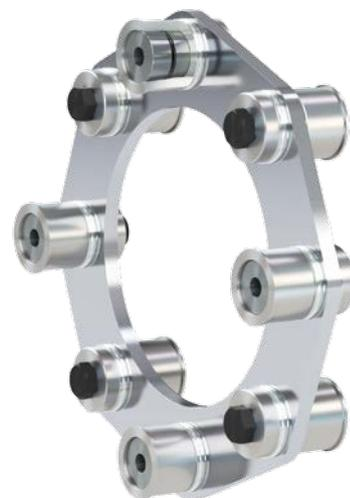
**For this backlash-free, positive locking connection, far lower screw tightening torques are required in comparison to standard frictionally locking connections. This makes installation substantially easier. The shape of the disks is FEM-optimised.**
