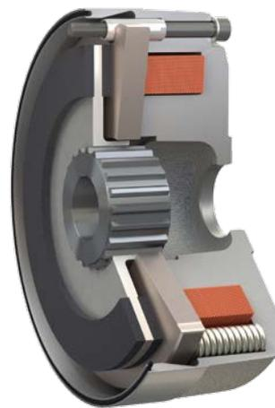
The ROBA-stop®-M safety brakes are designed for adverse ambient conditions. They are completely enclosed around the outer diameter and comply with Protection IP54 in standard design. Increased protection types are thus easily realisable. They cover a braking torque range from 2 to 1,600 Nm.
