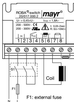
The power circuit is interrupted between the rectifier and the coil as well as mains-side. The magnetic field reduces extremely quickly. This causes a quick rise in braking torque.
