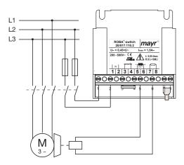
AC-side switching means **low-noise switching**; however, the brake engagement time is longer (approx. 6-10 times longer than with DC-side switching), use for non-critical braking times.
