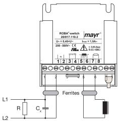
Measures against interference may prove unnecessary if suitable measures are already present in the system (shielded lines, shielding housing, appropriate wiring, etc.).
