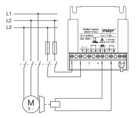
DC-side switching means short brake engagement times (e.g. for EMERGENCY STOP operation); but louder switching noises will occur.
