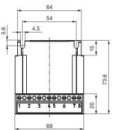
Accessories: Mounting bracket set for 35 mm rail acc. EN 60715: Article No. 1802911
