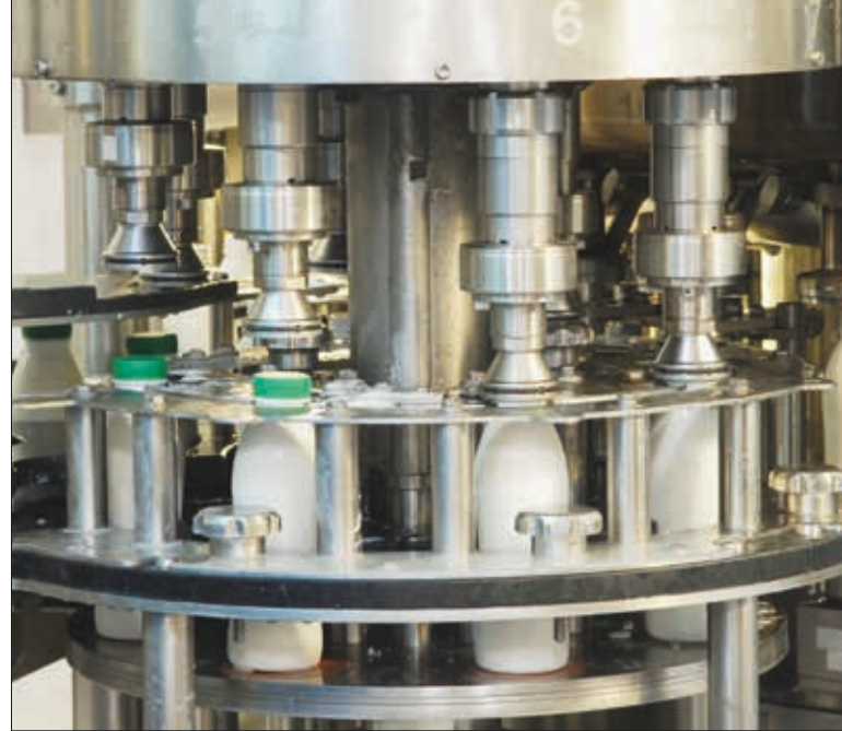
A filling line for drinking yoghurt: the hysteresis clutch, with its constant and shock-less capping torque, is particularly suitable for applying plastic screw caps with a preformed thread. (Picture: mayr® Antriebstechnik)
